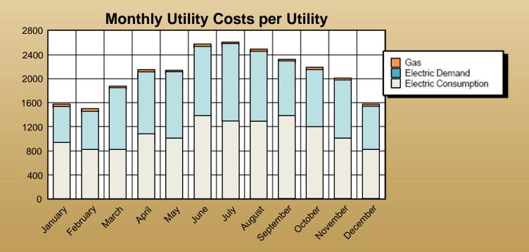
The chart above shows the monthly breakdown of utility costs for the building. As expected, the gas costs are very minimal compared to the electric consumption and demand. If we compare the electric consumption with the chart on the previous page we can see it varies accordingly. The chart on the following page shows the local utility rates that were used in calculating the utility costs.
